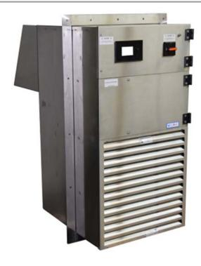
VoltAire Systems PU1600 Series Pressurization Units are designed to provide the ability to apply positive pressure to a building or room. Pressure levels are monitored by an internal controller that modulates airflow to maintain room/building pressurization. Filters prevent any potential dust or debris from entering the pressurized area.
